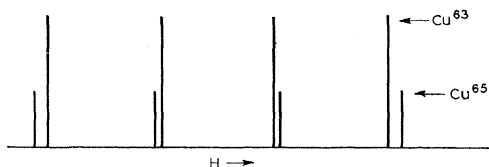
FIG. 5. An illustration of how the different moments of the two Cu isotopes broaden and lower the peak intensities of the two outer hfs components relative to the two center ones.
